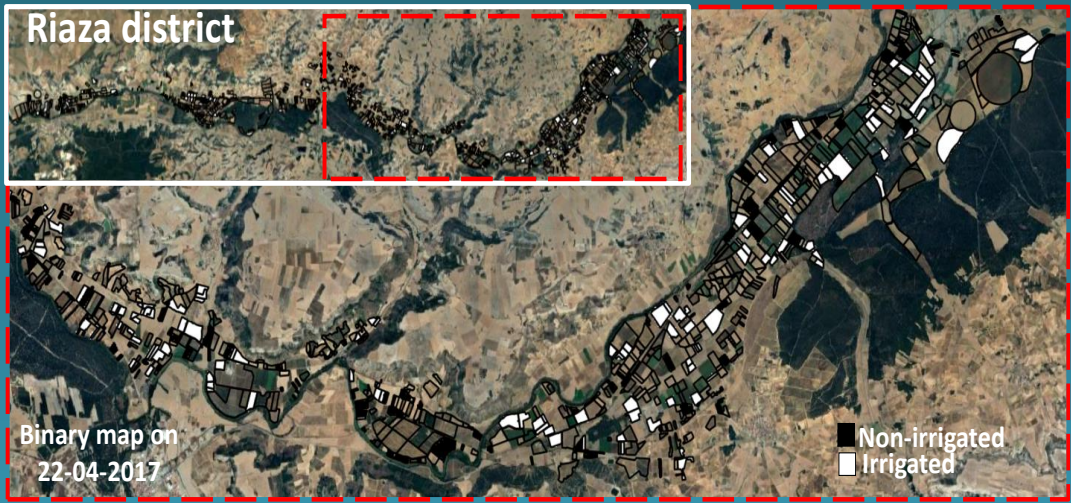
Example of irrigated/non-irrigated map, derived from EO SSM data over the Riaza irrigation district in Castilla y León region (Spain) on April 22, 2017. A zoomed-in view of the inset (red dashed rectangle) is shown
