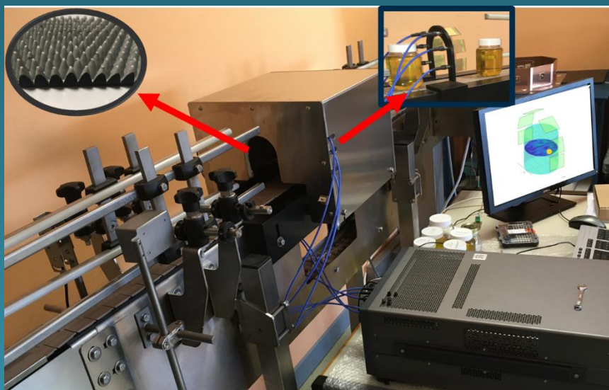
The MW imaging device developed by IREA researchers in collaboration with researchers from Politecnico di Torino in the framework of the BEST-FOOD project
